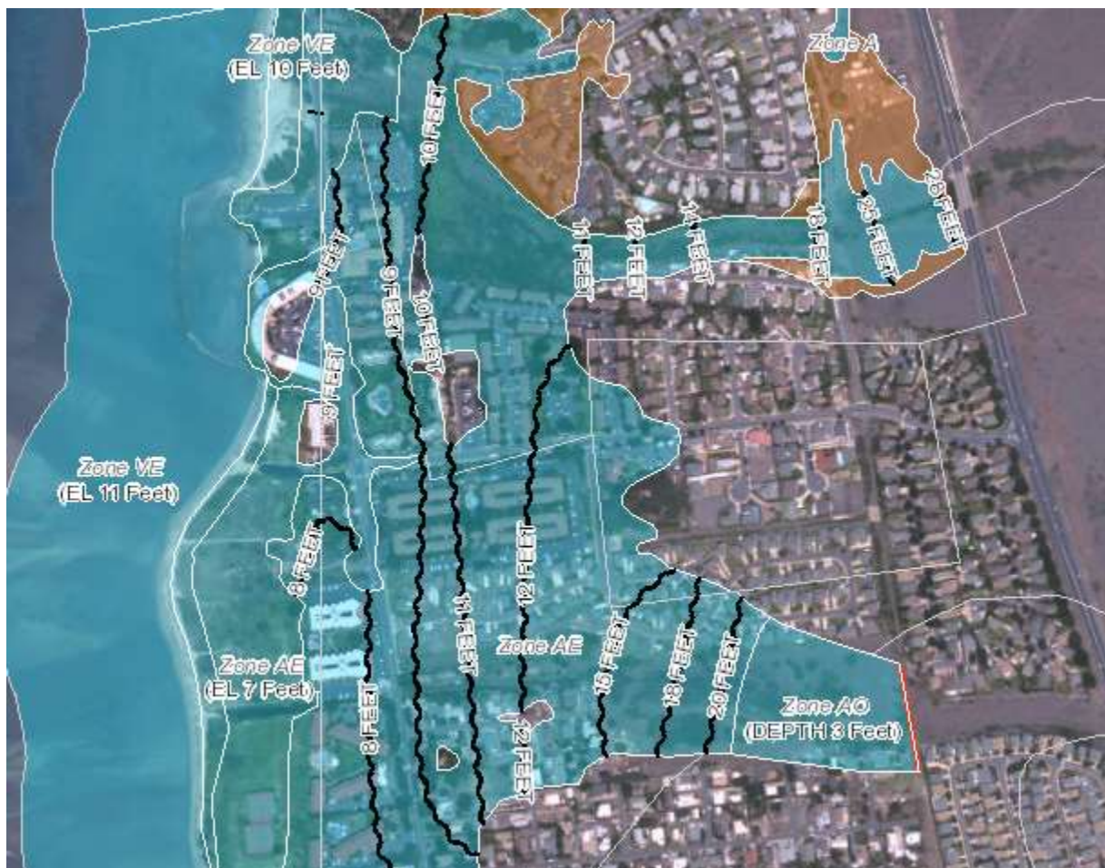
Figure 2. FEMA National Flood Hazard Layer map of the Kihei study area. The existing conditions 100-year flood model (unknown flood discharge) indicates significant flooding along South Kihei Road and overbank flooding along Waipuilani Gulch.
