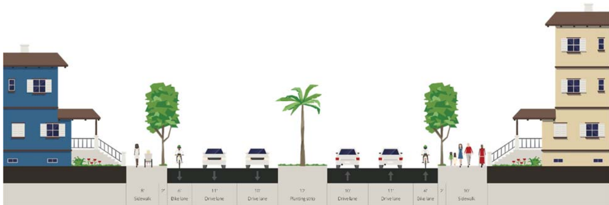
Figure 3-2: Parkway - Typical Cross Section (88-foot ROW)
